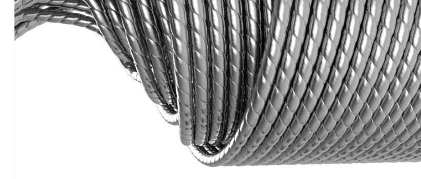
RAD shell and coil heat exchangers are perfect for installations where water from the ground heat source is fed directly into the exchanger. Larger internal diameter of the tubes makes it less prone to clogging than with brazed plate heat exchangers. A filter/strainer is still required to prevent ingress of debris and particles carried by the water. RAD exchangers are made entirely of high quality austenitic stainless steel, granting them a high resistance to corrosion.
