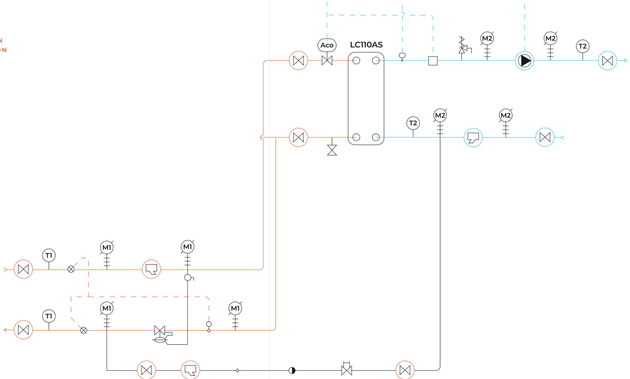
The task of a single-function district heating substation is transferring heat from a heating grid to the building's central heating grid through a plate heat exchanger. This allows to achieve a lower temperature and pressure in the system than in the heating grid, which is safer for the end user. Hexonic's extensive product range provides a selection of exchangers for district heating substations of virtually any size.
