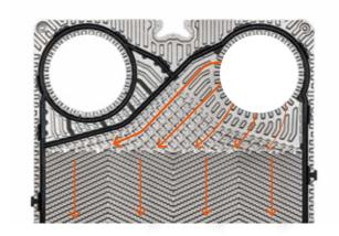
Additionally corrugated distribution area is designed to enhance turbulent flow in the entrance part of the plate. It also allows even flow through the plate which increases heat transfer by optimal use of its surface area.
